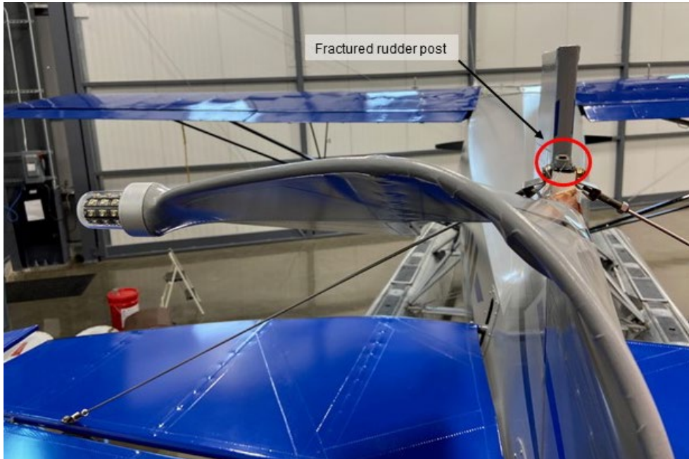
Figure 1. Photograph showing the fractured rudder post from N3188M (case number ANC20LA059).
