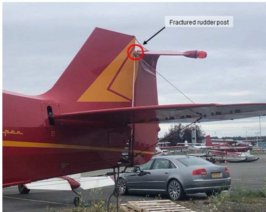
Figure 2. Photograph showing the fractured rudder post on N4206H (case number ANC21LA064).
